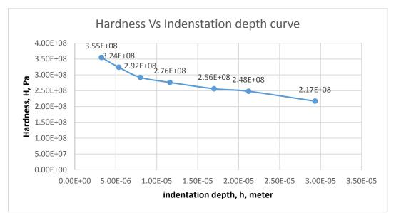
The density of geometrically necessary dislocations obtained from above hardness measurement values is  $1.81*10^{14}$  m<sup>-2</sup> whereas for the same sample dislocation density obtained from XRD experiments are  $1.2*10^{14}$  m<sup>-2</sup>.
