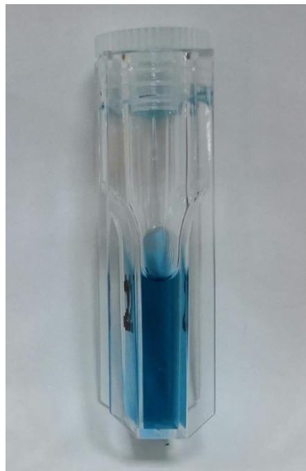
Figure 5: A photograph of the irradiated sample (Cuvette) of 0.1 mM Fricke-MTB gelatin dosimeter system by Am-243.
