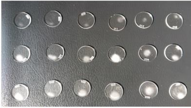
Figure 1. Detectors exposed to a Ra-223 activity of 10 kBq
