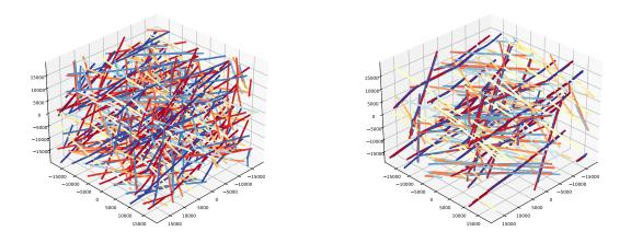
Figure 1: An initial configuration of a single loop and its periodic images (left) and the nearly relaxed systems (right). The displayed region is the simulation cell including the dislocation lines. Colours indicate the type of the dislocation: red and blue (according to the conventional colouring of 2D) are edge dislocation segments and yellow is screw dislocation segment. The right panel confirms the formation of narrow dipoles in this 3D system.
