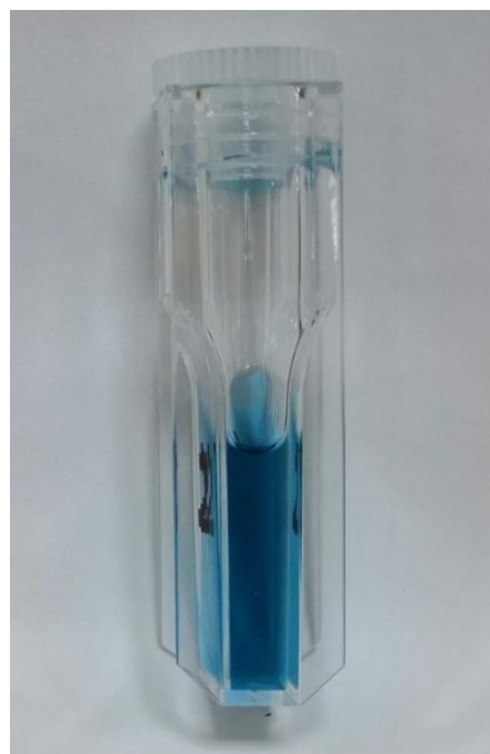
Figure3: A photograph of the irradiated sample (Cuvette) of 0.1 mM Fricke-MTB gelatin dosimeter system by Am-243.
