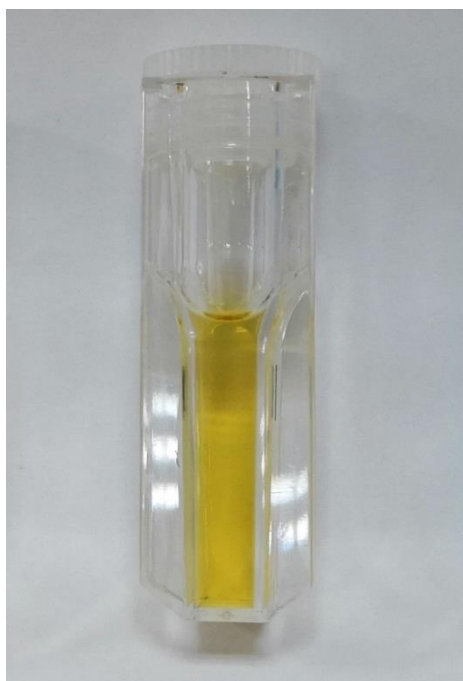
Figure2: A photograph of the unirradiated sample (Cuvette) of 0.1 mM Fricke-MTB gelatin dosimeter system.
