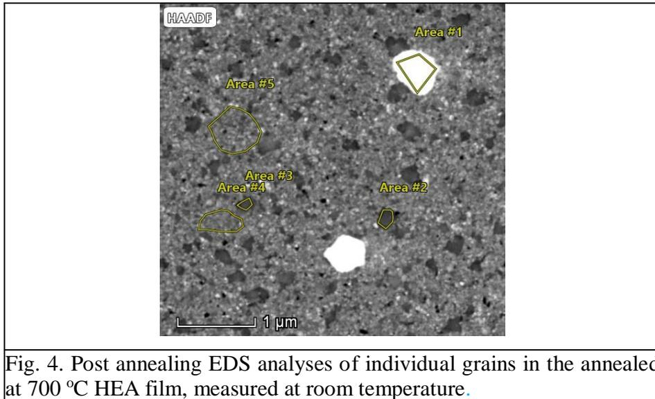
Fig. 4. Post annealing EDS analyses of individual grains in the annealed at 700 °C HEA film, measured at room temperature.
