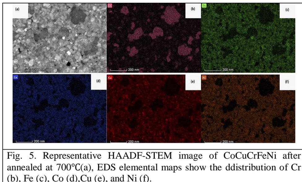
Fig. 5. Representative HAADF-STEM image of CoCuCrFeNi after annealed at 700°C(a), EDS elemental maps show the distribution of Cr (b), Fe (c), Co (d), Cu (e), and Ni (f).
