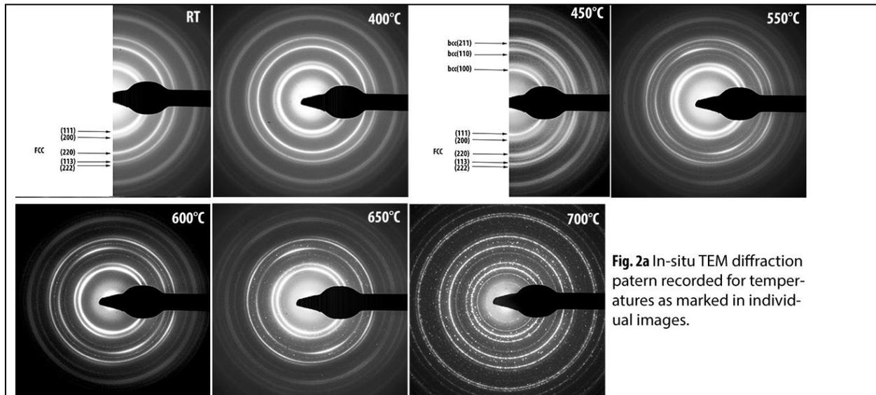
**Fig. 2a** In-situ TEM diffraction pattern recorded for temperatures as marked in individual images.
