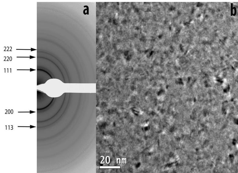
Fig. 1. Electron diffraction pattern (a) Bright field TEM image (b) of the HEA film before annealing. Electron diffraction indicates a single fcc phase.
